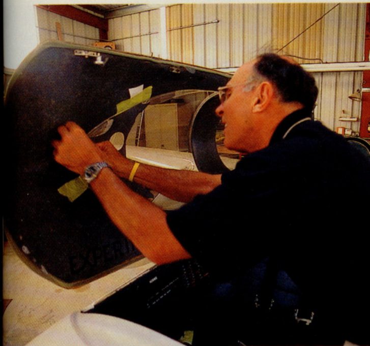
SpaceShipOne pilot Mike Melvill (above) flew simulated flights in his Long EZ in preparation for the actual flight in SpaceShipOne. To replicate the limited forward visibility in SpaceShipOne, Melvill covered the inside of the Long EZ canopy with cardboard (above), which had four small holes cut into it, mimicking the spacecraft's cockpit.
