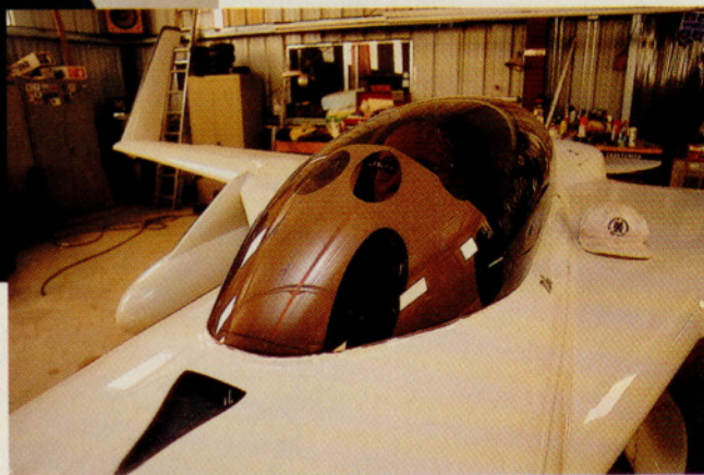
SpaceShipOne pilot Mike Melvill (above) flew simulated flights in his Long EZ in preparation for the actual flight in SpaceShipOne. To replicate the limited forward visibility in SpaceShipOne, Melvill covered the inside of the Long EZ canopy with cardboard (above), which had four small holes cut into it, mimicking the spacecraft's cockpit.
